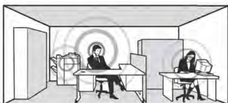
Room with sound absorption through acoustically treated furniture, floor and ceiling
