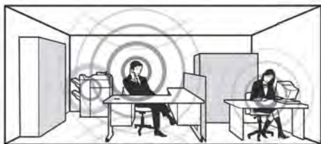
Room with sound absorption through acoustically treated office furniture
